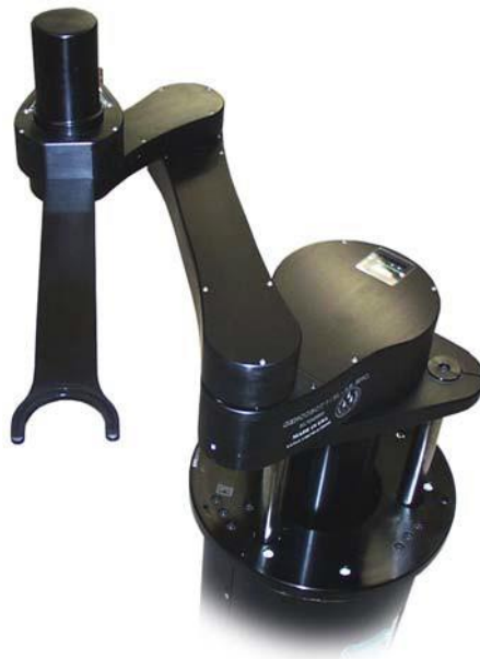
Figure1. A six-DOF GPR robot with “yaw-axis” capabilities
