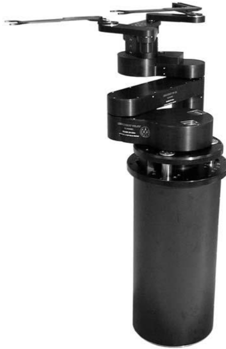
Figure 2. A fast-swapping robot, capable of handling four 300 mm in-line FOUPs
